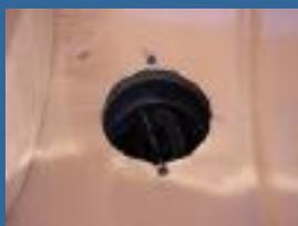
I drilled out two holes and mounted the vent. Then marked and cut out the damper opening. Once again I put the top barrel back on the bottom to check fit the collar.
