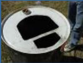
Here is the opening for the fire door once it is cut out. I needed to use a file to make the two holes a little larger, I didn't want to risk making them to big with the saw. Once you have the door in then just drill out the holes and bolt it in. As you will see in other photos it goes on easy.
