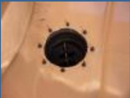
Here is the final mounting of the vent damper. You will need to do this on the other end of the barrels as well. You can follow these instruction for the other lower vent damper.
